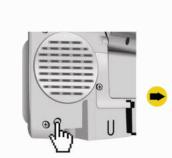
Execute the hard reset by pressing the Reset button as shown left.
